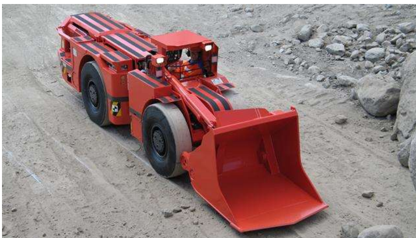
Fig. 1. Overall view of the loading, transporting and storing machine, model TORO 151 produced by Sandvik
