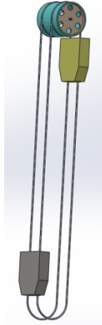
Fig. 3. Assembly of statically balanced multi-rope hoisting machinery. The fully loaded transportation container is on the ascending arm
