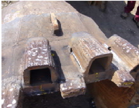
Fig. 6. Renewed cutting blade with adapters
