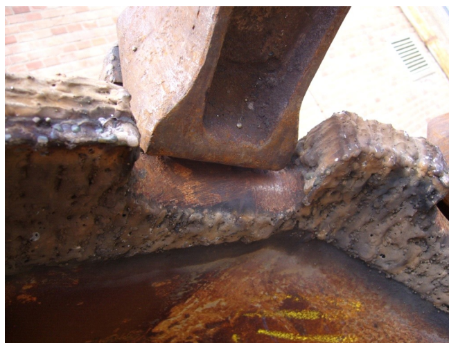
Fig. 3. The deficiency of the relative position of the tooth on cutting blade at the renewed buckets
