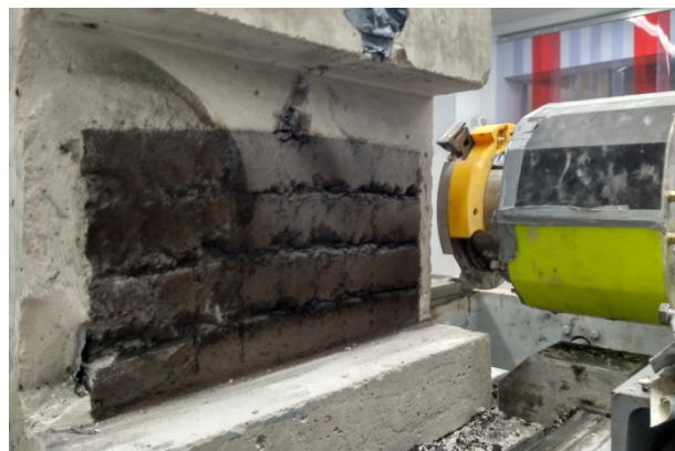
Fig. 2. Rotary cutting test bench on starting position before cutting an artificial boundary of coal and host rock.
