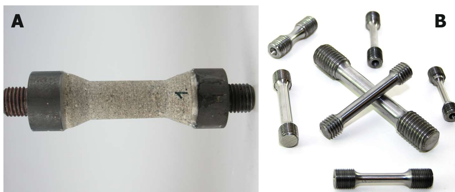
Figure 1. A - rotational symmetric AWJ formed sandstone specimen prepared for tensile strength testing, B - specimens used for testing of uniaxial tensile strength of metals
